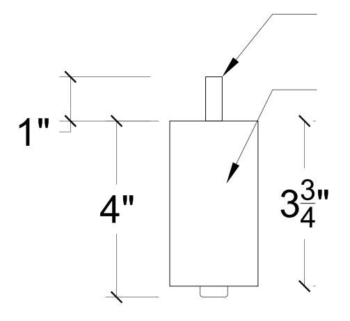
STEEL WOOD SCREW THREADED STUD. (THREADED SIZE 5/16-18)
